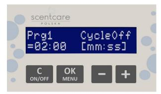
ProSense is now ready to work! Scheduled programs will be applied after approx. 20 seconds (you can also exit the Main Menu by pressing button). Please keep in mind that the device will prioritize programs by its order. That means, if you will set up more than 1 program for Wed and Sat, ProSense will only use the schedule from the 1<sup>st</sup> one. Avoid scheduling the same time periods in different programs.
