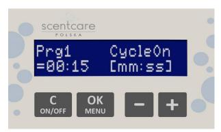
Flashing timer means you can set up the duration of the scent dosing with 🛨 🖃 buttons.
